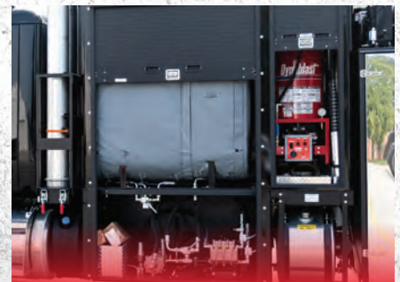
Insulated Enclosure Houses Blower & Water Pump
